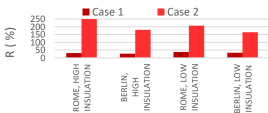
Fig. 12 - SW exposure. Relative increase on heating demand
