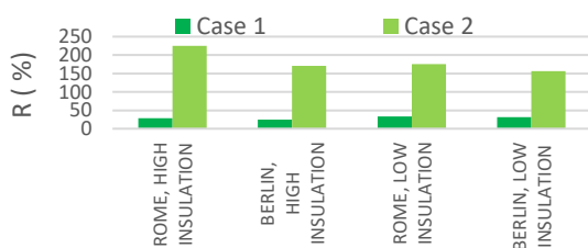
Fig.11– NE exposure. Relative increase on heating demand
