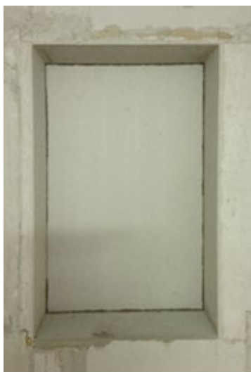
Fig. 2 – Installation of the panel according to ISO 10140
