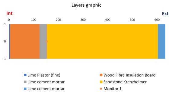
Fig. 1 – Graphical visualization of the layers constituting the building element and of the monitor position within the GUI of ProCasaClima Hygrothermal
