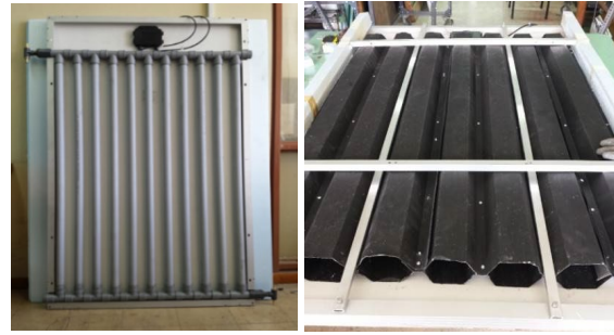
Fig. 2 – Water (left) and air (right) PVT heat extraction systems
