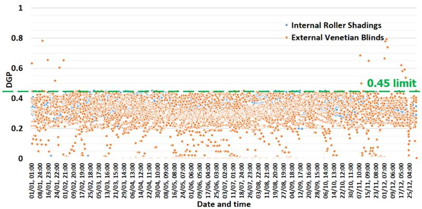
Fig. 6 – Daylight Glare Probability with the two systems
