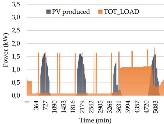
Fig. 6 – PV produced power and system's load for the standard HVAC strategy, from 15th to 19th of January
