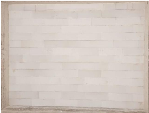
Fig. 5 – Wall – Laboratory test according to ISO 10140 (2021) series standard
