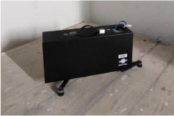
Fig. 1 – Investigated CLT floor mechanically excited using a standardized tapping machine
