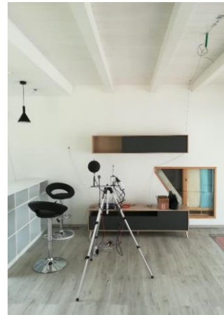
Fig. 2 – Sensors and instruments installed in the central room of the building prototype
