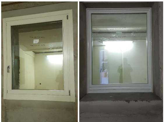
Fig. 3 – Window – Laboratory test according to ISO 10140 (2021) series standard
