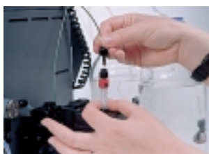
Connecting the column.
