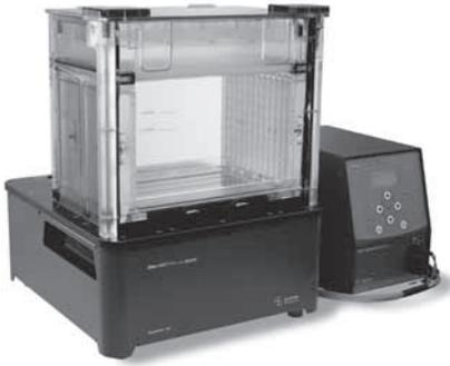
Fig 3. Ettan DALTwelve Large Vertical System.
