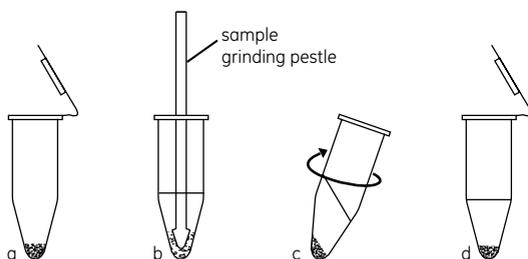
**Fig 8.** Schematic of the method used in the Sample Grinding Kit. (a) Pellet grinding resin in microcentrifuge tube. (b) Add sample and extraction solution. Disrupt sample by grinding with pestle. (c) Centrifuge to separate cellular debris and resin. (d) Collect supernatant.
