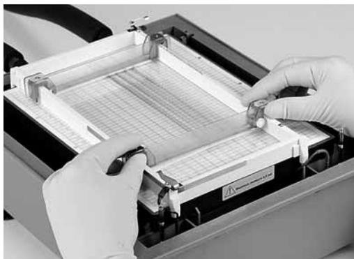
Fig 49. Alignment of electrodes over Immobiline DryStrip gels.
