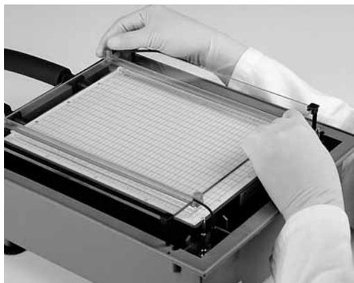
Fig 56. Positioning electrodes.
