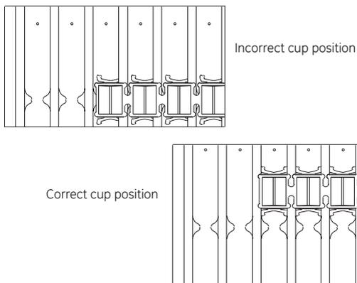
**Fig 31.** Sample cup positioning details.
