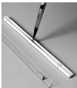
**Fig 26.** Applying rehydration solution into the Strip Holder.
