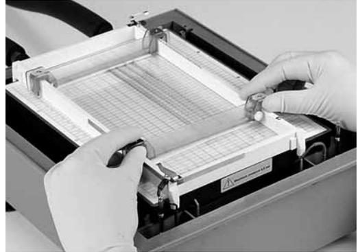
Fig 49. Alignment of electrodes over Immobiline DryStrip gels.
