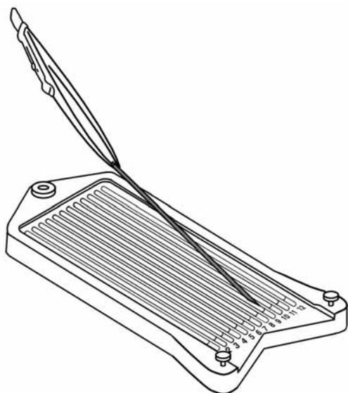
**Fig 47.** Positioning an Immobiline DryStrip gel in the Immobiline DryStrip Reswelling Tray.
