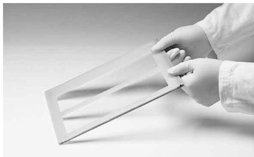
**Fig 38.** Closing the DALT Precast Gel Cassette.
