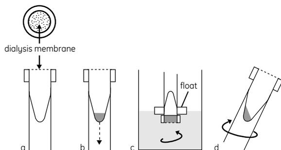
**Fig 11.** Schematic of the method used in Mini Dialysis Kit. (a) Cap with dialysis membrane, conical inner sample tube. (b) Introduce sample, screw on cap, and slide tube into float. (c) Invert and dialyze while stirring. (d) Spin briefly to collect sample.
