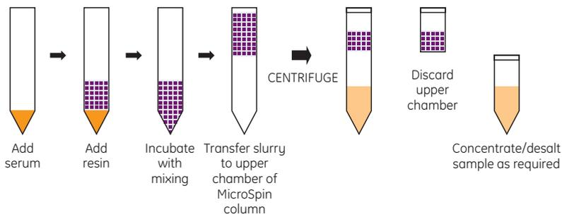
**Fig. 14.** Schematic of the removal process. Optimal albumin and IgG binding (>95% total protein) is achieved using a 15  $\mu$ l human serum loading and will typically lead to recovery of between 150 and 220  $\mu$ g of lower-abundance proteins. The amount of protein recovered will vary with the protein content of the individual serum samples used.
