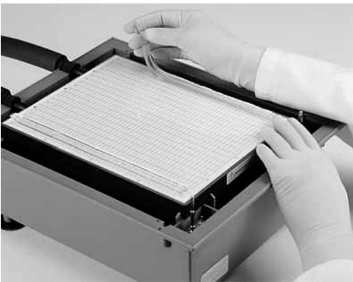
Fig 53. Positioning the anodic buffer strip on Multiphor II unit.
