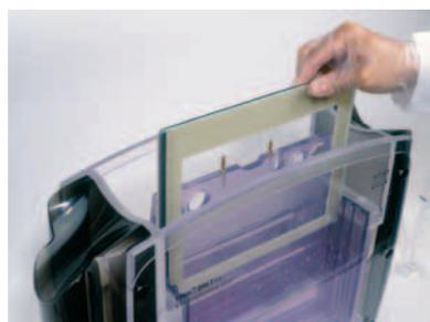
**Fig 42.** Inserting the cassettes into the cassette carrier.
