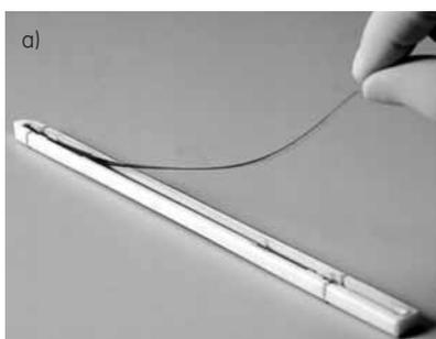
**Fig 27. a, b.** Positioning the Immobiline DryStrip gel.
