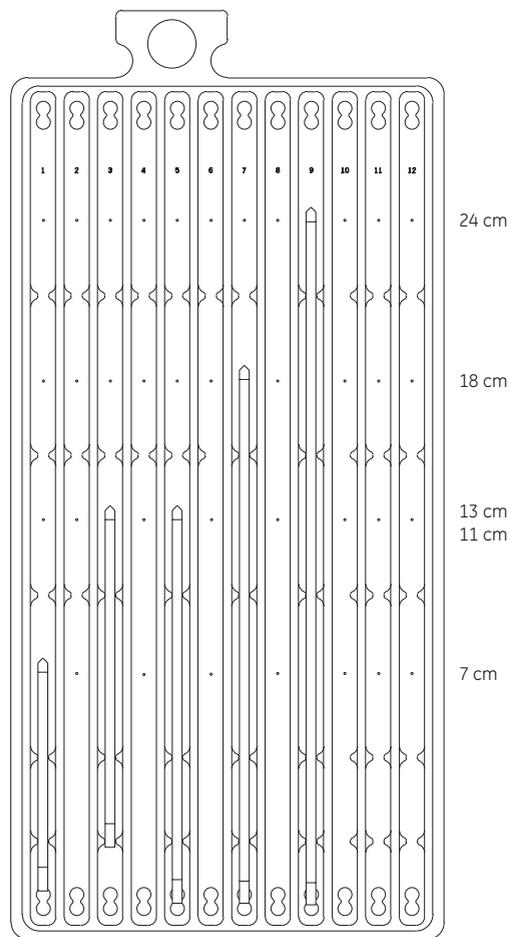
**Fig 30.** Placement of IPG strips in Manifold channels.
