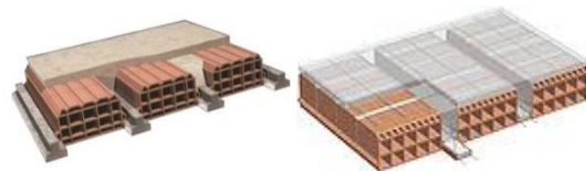
Fig. 4 – Examples of considered structural roofs. a) precast concrete and prestressed reinforced, b) traditional masonry
