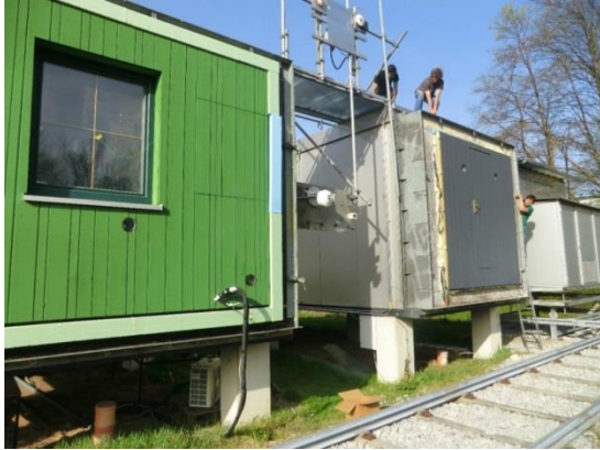
Fig. 5 – PASSYS test cell at UIBK with installed functional models, left cell: 1st functional model (MVHR next to window), right cell: 2nd functional model (μHP and MVHR) – photo: UIBK
