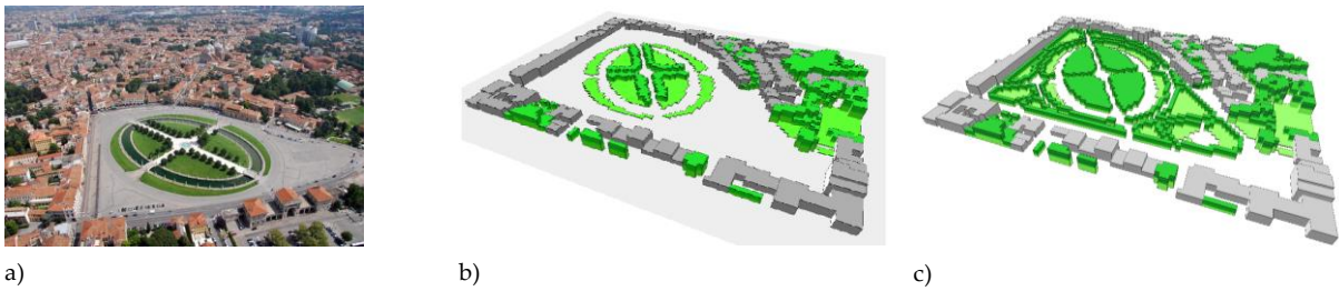
Figure 1 – The area (a) and the model area in ENVI-met used for the simulations of the “AsIs” scenario (b) and the “Green ground” scenario (c)
