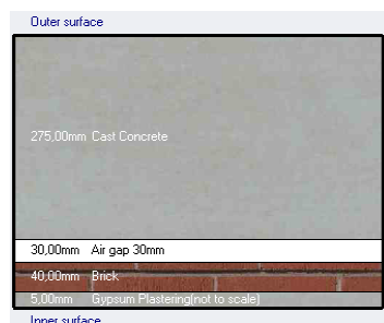
Fig. 4 – Drawing of the external wall construction
