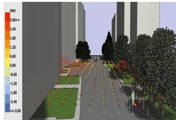
Fig. 3 – The 3-Dimension visualization of PMV vectors (z)
