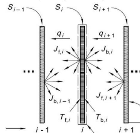
Fig. 3 – Layer-by-layer modelling according to ISO15099
