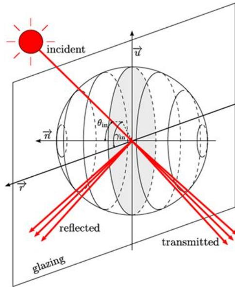
Fig. 4 – Optical modelling with BSDF data
