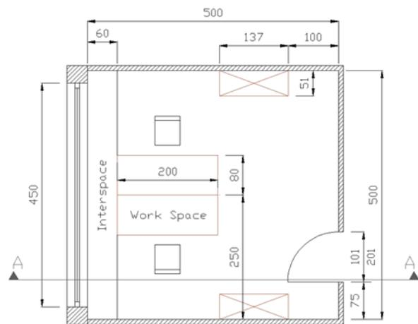
Fig. 5 – Dimensions of the double-office reference room
