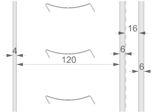
Fig. 7 – Geometrical definition [mm] spec. in-between blind „Alar“
