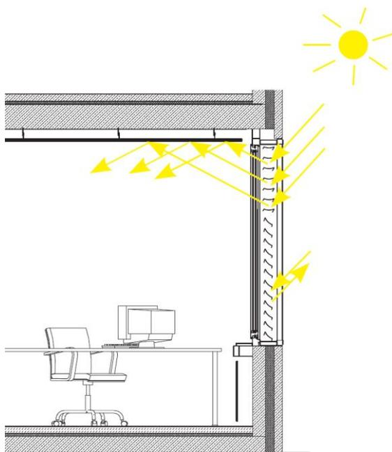
Fig. 1 – Light redirecting facade system
