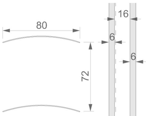
Fig. 6 – Geometrical definition [mm] - external raffstore „RAF“
