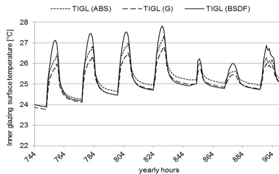
Fig. 9 – Inner glazing temperature (Raffstore) - winter condition
