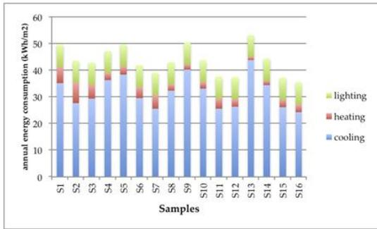
Fig. 2 - HVAC and lighting performance of optimum samples
