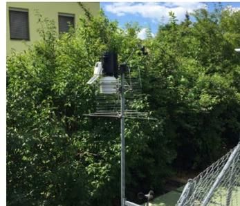
Fig. 8 – Wireless local weather station
