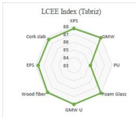
Fig. 9 – Life cycle energy efficiency index for different insulation scenarios in Tabriz
