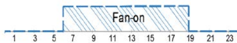
(a) The ventilation system of the façade cavity was on all year during working hours only.
