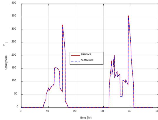
Fig. 5 – Comparison of the incident solar radiation, per surface unit, on a vertical South wall, obtained with TRNSYS and ALMABuild
