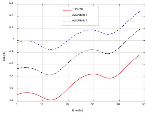
Fig. 4 – Comparison of the room air temperature considering radiative heat exchange, with the same  $T_{sky}$  used in TRNSYS, (ALMABuild 2) and with a different  $T_{sky}$ , ALMABuild 1
