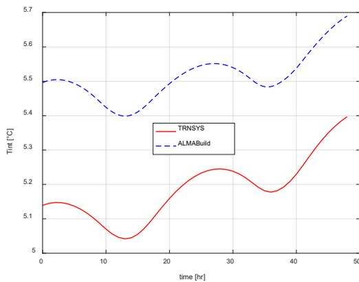
Fig. 7 – Comparison of the room air temperature, considering all the thermal fluxes on the opaque component, with TRNSYS and ALMABuild
