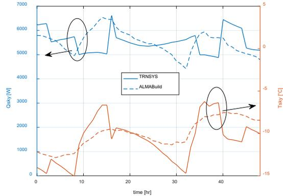
Fig. 2 – Comparison of the radiative heat exchange with the sky (left side, upper lines) and effective temperature of sky (right side, lower lines) obtained with ALMABuild (dashed line) and TRNSYS (solid line)
