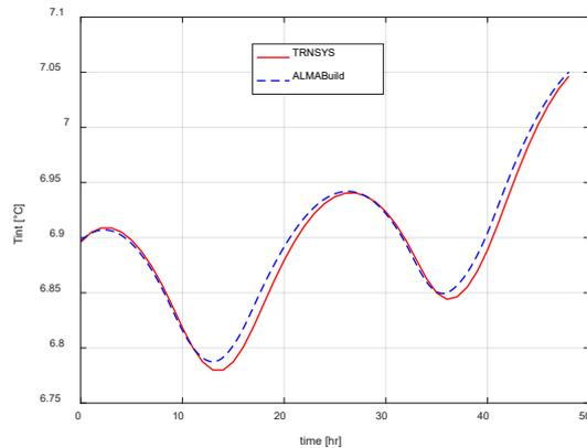
Fig. 6 – Comparison of the room air temperature, considering solar heat gains, with TRNSYS and ALMABuild
