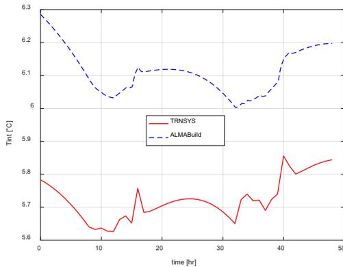
Fig.9 – Comparison of the room air temperature, considering the thermal zone with a window, obtained with TRNSYS and ALMABuild
