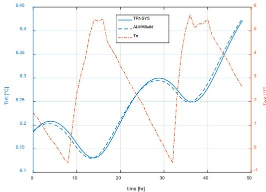
Fig. 1 – Comparison of the room air temperature ( $T_{int}$ ) obtained with ALMABuild (dashed line) and TRNSYS (solid line)
