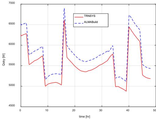
Fig. 3 – Comparison of the radiative heat exchange with the sky obtained with ALMABuild and TRNSYS, using the same  $T_{sky}$
