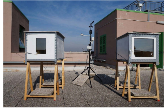
Fig. 1 – STBs with different window frames during the calibration test
