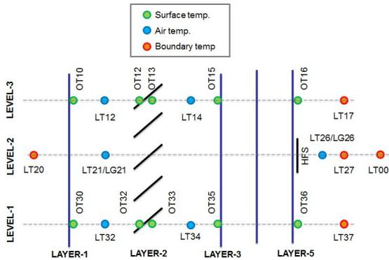
Fig. 5 – Sensor positions on the three measuring levels
