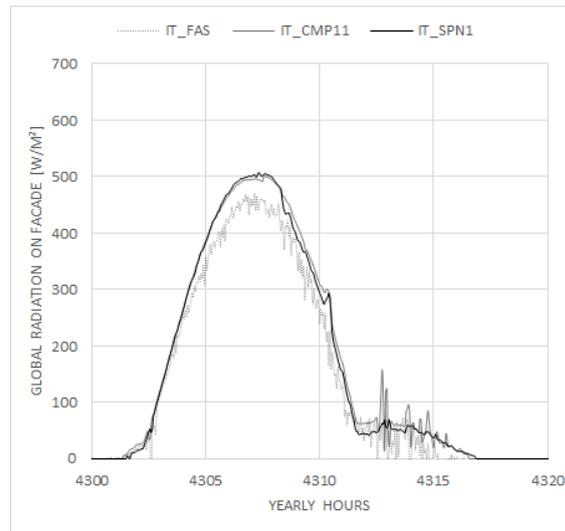
Fig. 6 - Irradiance on Façade: measured vs. simulated
