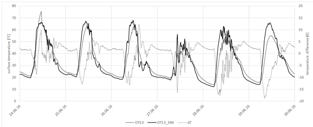
Fig. 9 – Blind temperature, System 2 - 0° slat angle
