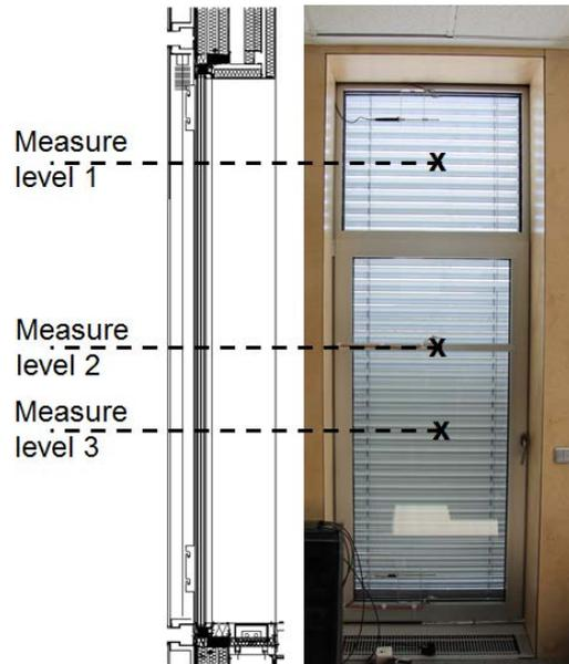
Fig. 4 – Height levels of measurement at the test façade
