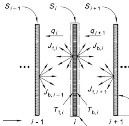
Fig. 2 – Layer-by-layer modelling according to ISO 15099
