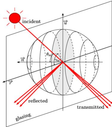
Fig. 1 – Thermal modelling of transmitted solar gains by BSDF datasets (Hiller and Schöttl, 2014)
