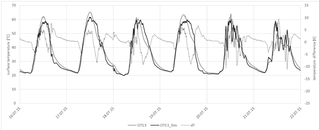
Fig. 8 – Blind temperature, System 1 - 45° slat angle
