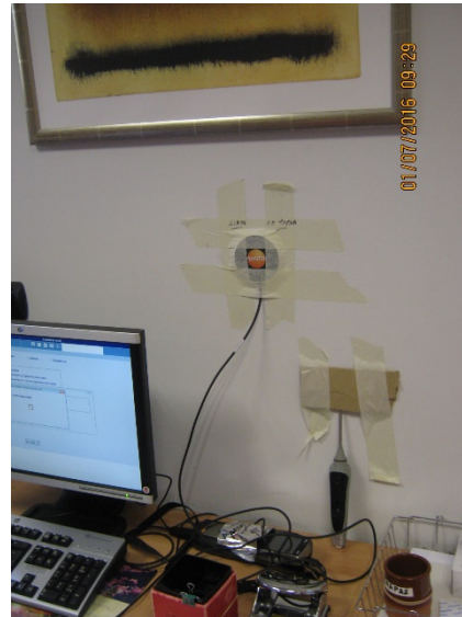
Fig. 4 – Internal measurement equipment for heat flow rate, surface temperature, and air temperature (Passerini, 2016)
