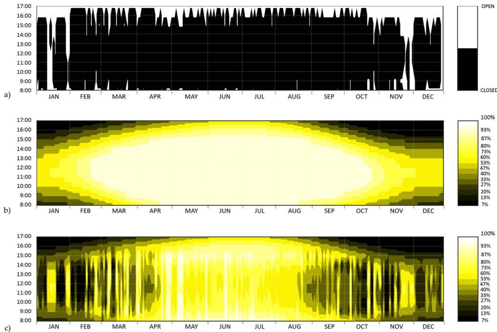
Fig. 1 – Temporal plot for the shades' opening percentage according to CTRL1 (a), 2 (b) and 3 (c) for the small window S1, with HH glazing system
