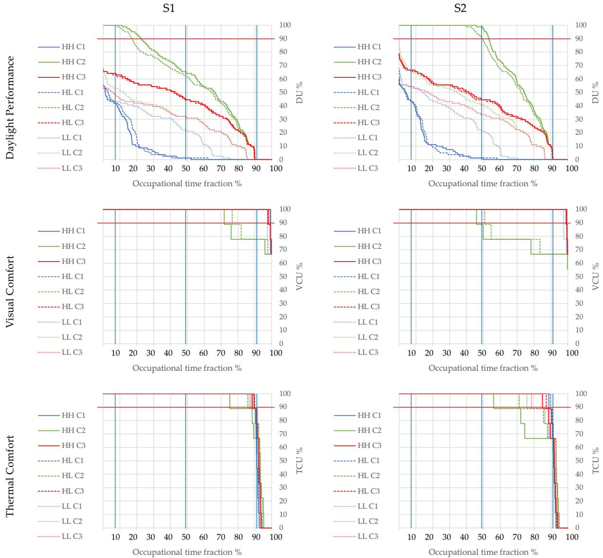
Fig. 3 – Daylight Usability, Visual Comfort Usability, and Thermal Comfort Usability for small and large windows
