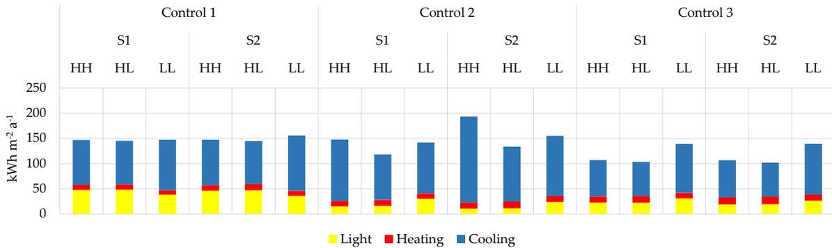
Fig. 4 – Primary Energy demand for artificial lighting, heating and cooling
