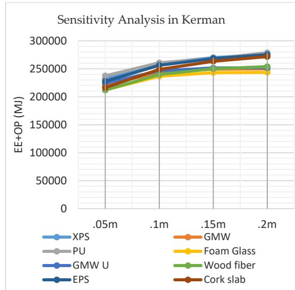
Fig. 4 – Sensitivity analysis of insulation thickness and total energy demand in Kerman
