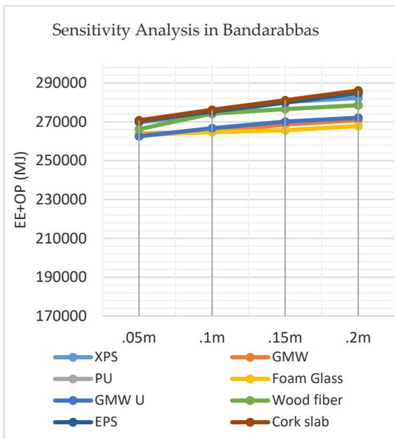
Fig. 3 – Sensitivity analysis of insulation thickness and total energy demand in Bandar Abbas
