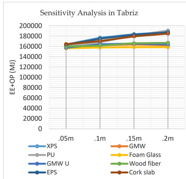
Fig. 5 – Sensitivity analysis of insulation thickness and total energy demand in Tabriz
