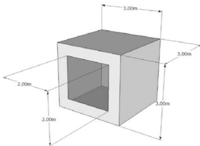
Fig. 1 – The thermal zone which is modeled in EnergyPlus 8.3
