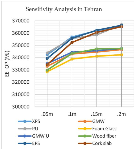
Fig. 2 – Sensitivity analysis of insulation thickness and total energy demand in Tehran
