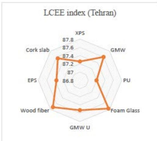
Fig. 6 – Life cycle energy efficiency index for different insulation scenarios in Tehran
