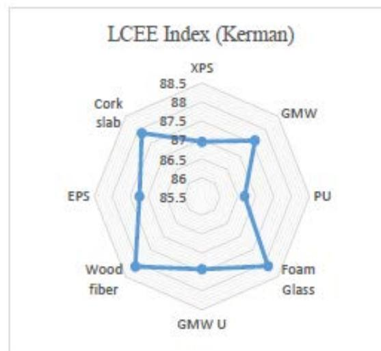
Fig. 8 – Life cycle energy efficiency index for different insulation scenarios in Kerman
