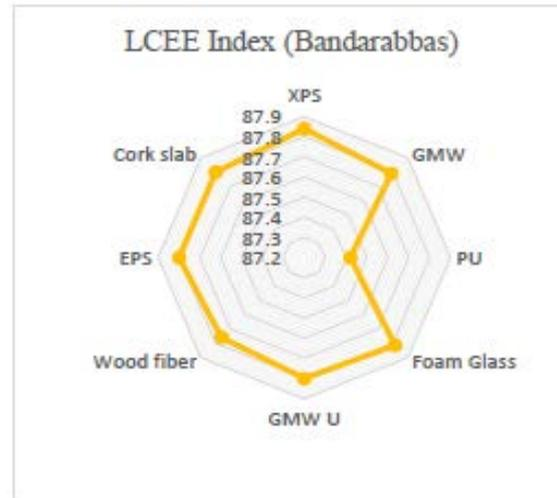
Fig. 7 – Life cycle energy efficiency index for different insulation scenarios in Bandar Abbas
