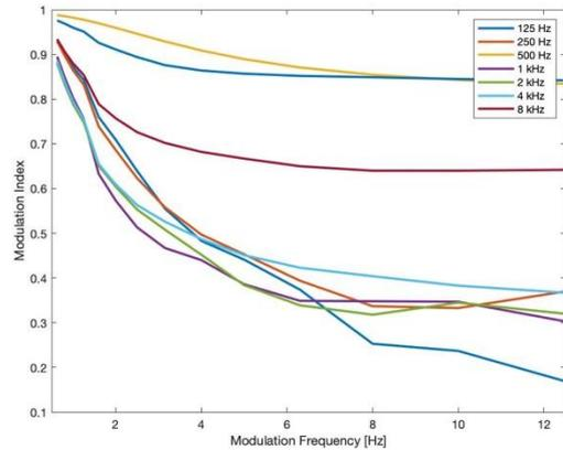
Fig. 5 – Modulation transmission ratio in the 7 octave bands
