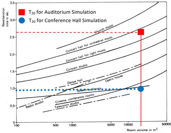
Fig. 8 – Optimal T<sub>20</sub> values at 500 Hz, based on room volume
