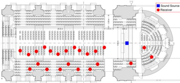
Fig. 4 – Equipment positions during the acoustic survey
