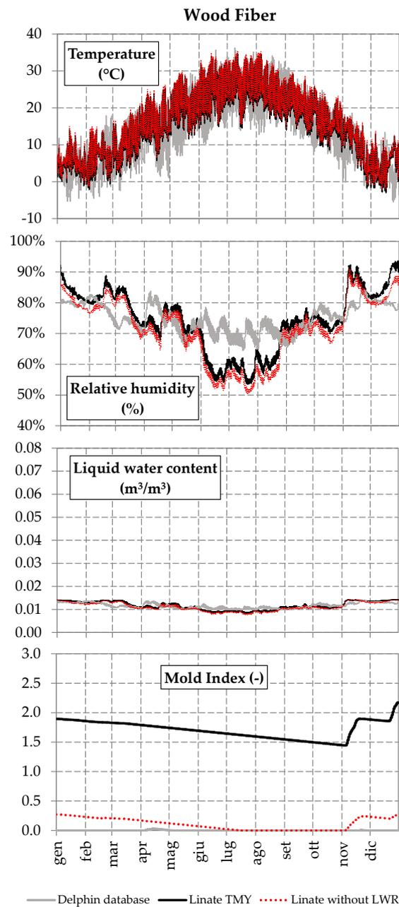
Fig. 4 – Comparison between simulations with weather data from Delphin database and Linate TMY with/without LWR
