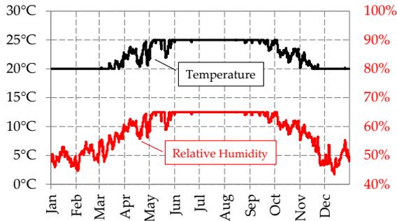
Fig. 2 – Indoor climate conditions as a function of outdoor temperature from Linatè TMY, according to EN ISO 15026 (CEN, 2007b)
