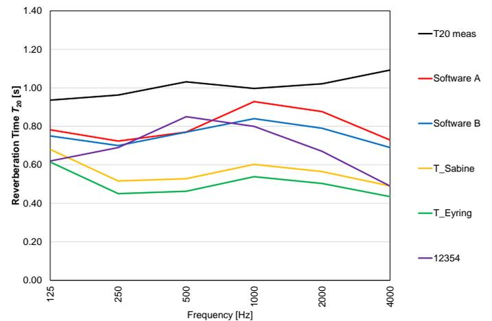
Fig. 11 – Measured and simulated reverberation time  $T_{20}$  (Room 2)
