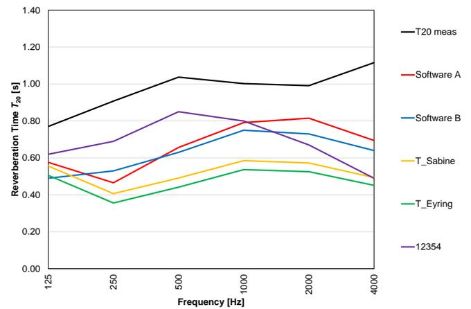
Fig. 10 – Measured and simulated reverberation time  $T_{20}$  (Room 1)
