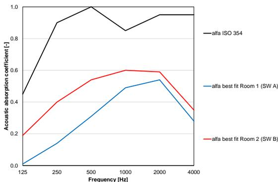
Fig. 16 – Best fit acoustic absorption coefficient
