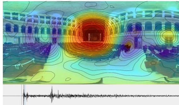
Fig. 15 – Acoustic map showing direct sound arriving to the receiver placed in the stalls
