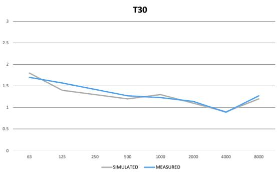
Fig. 9 – Reverberation time measured after reconstruction compared with the values obtained during the acoustic design in 2010
