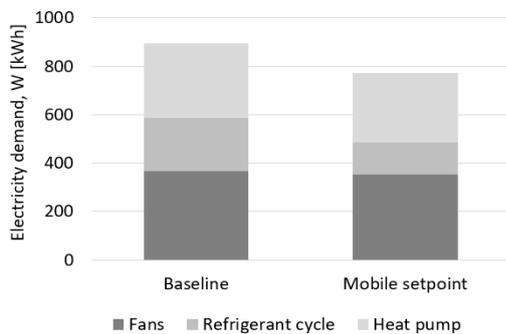
Fig. 5 – Electrical consumption during the cooling season
