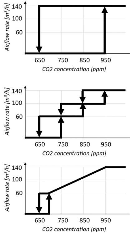
Fig. 3 – CO<sub>2</sub>-based DCV with on-off hysteresis (top), multistep modulation (middle) and proportional modulation (bottom)
