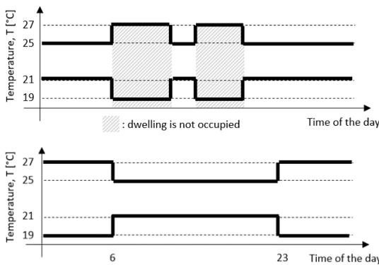
Fig. 4 – Temperature setpoints with non-occupancy setbacks (top) and night setbacks (bottom)
