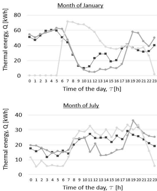
Fig. 8 – Hourly averages of heat pump energy generation
