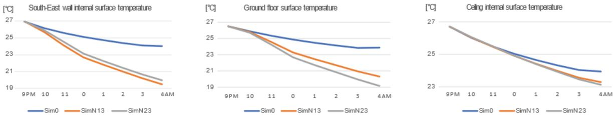
Fig. 5 – Nighttime natural ventilation simulations results: internal surface temperatures of different building components (4<sup>th</sup> of July)
