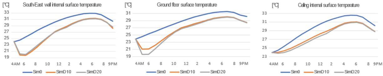
Fig. 4 – Daytime natural ventilation simulations results: internal surface temperatures of different building components (4<sup>th</sup> of July)
