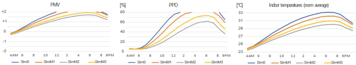
Fig. 6 – Thermal mass simulations results: PMV (a), PPD (b) and indoor temperature (c) trends (4<sup>th</sup> of July)
