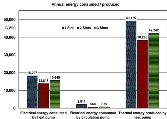
Fig. 5 – A comparison between annual energy consumed/produced in various activation time slots of the circulating pump
