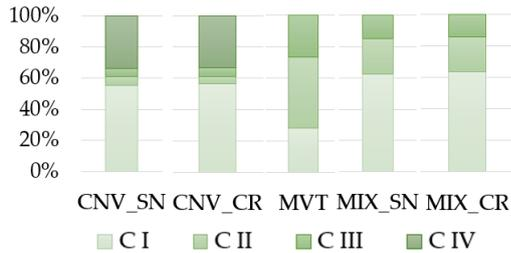
Fig. 2 – Distribution of IAQ categories (C I-C IV) for the CO<sub>2</sub> concentration during the occupied hours considering the five ventilation strategies during the summer period (May-September)
