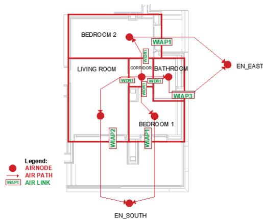
Fig. 1 – Reference building plan, thermal zones, airflow network
