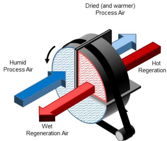
Fig. 1 – Diagram of a desiccant wheel
