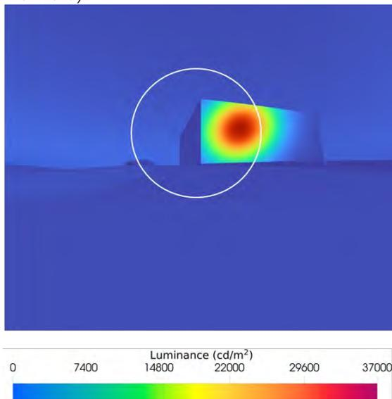
Fig. 4 – Winter solstice morning solar reflection off east facade glazing. View based luminance rendering at roadway viewing position
