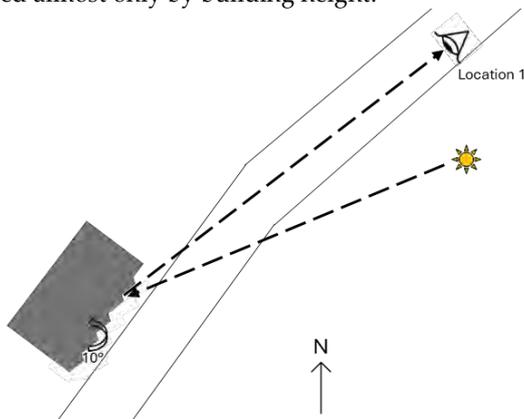
Fig. 6 – Perpendicular reflection example – mitigation by glazing reorientation
