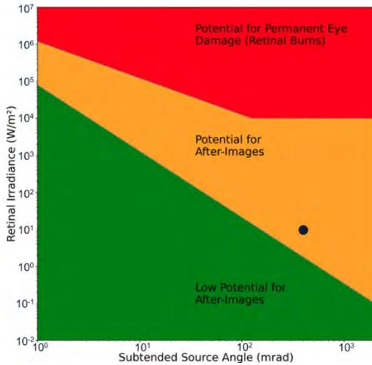
Fig. 3 – Potential impacts of retinal irradiance vs subtended source angle criteria by Ho et al. Result for winter solstice morning solar reflection off east facade glazing at roadway viewing position
