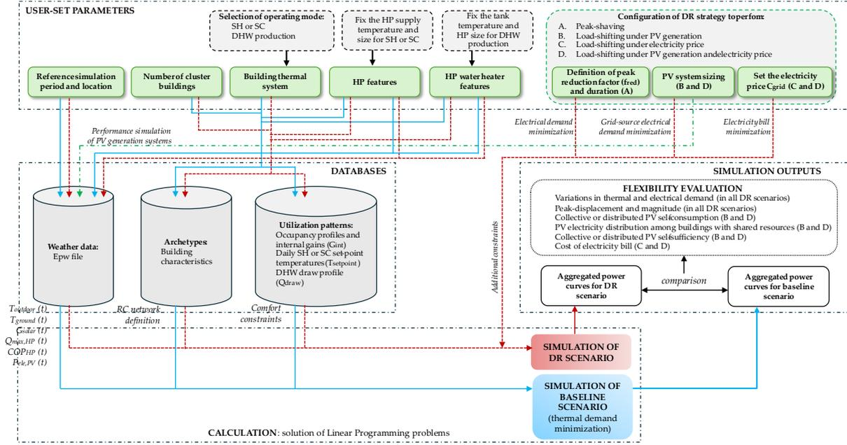
Fig. 1 - Schematic of ClustEnergy OpTool operation
