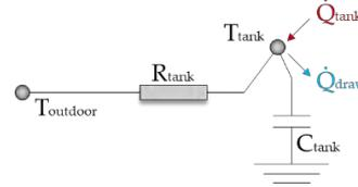
Fig. 3 – RC network model of a heat pump water heater
