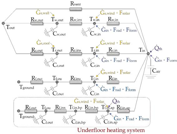
Fig. 2 – RC network model of a thermally insulated building with air emission system ( $Q_{th}$  applied to the indoor air thermal node) and underfloor heating system ( $Q_{th}$  applied to the innermost thermal node of the floor)
