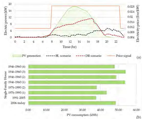
Fig. 4 – (a) Aggregate electric power trends for SC and DHW production during baseline and DR scenarios and (b) distribution of PV electricity among cluster buildings during DR scenario
