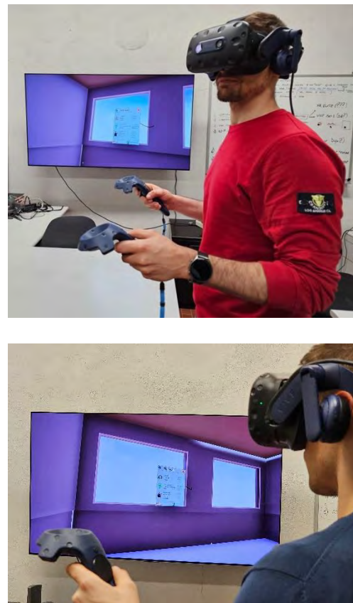
Fig. 6 – The implemented virtual reality environment for testing the proposed procedure. The user is wearing a HTC Vive Pro 2 helmet
