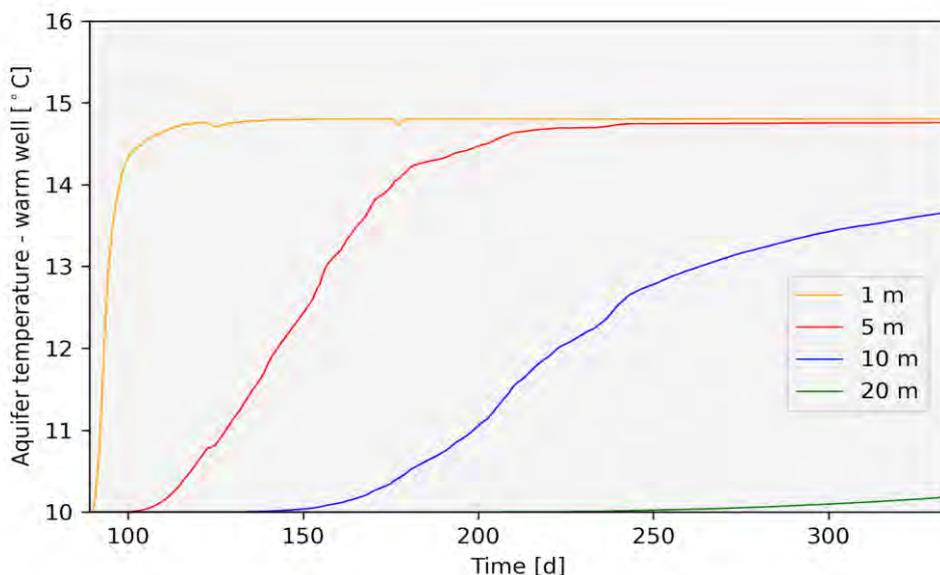
Fig. 5 – Temperature in the warm well of the aquifer at different distances
