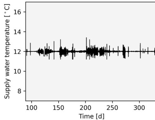
Fig. 4 – Supply water temperature to hospital buildings
