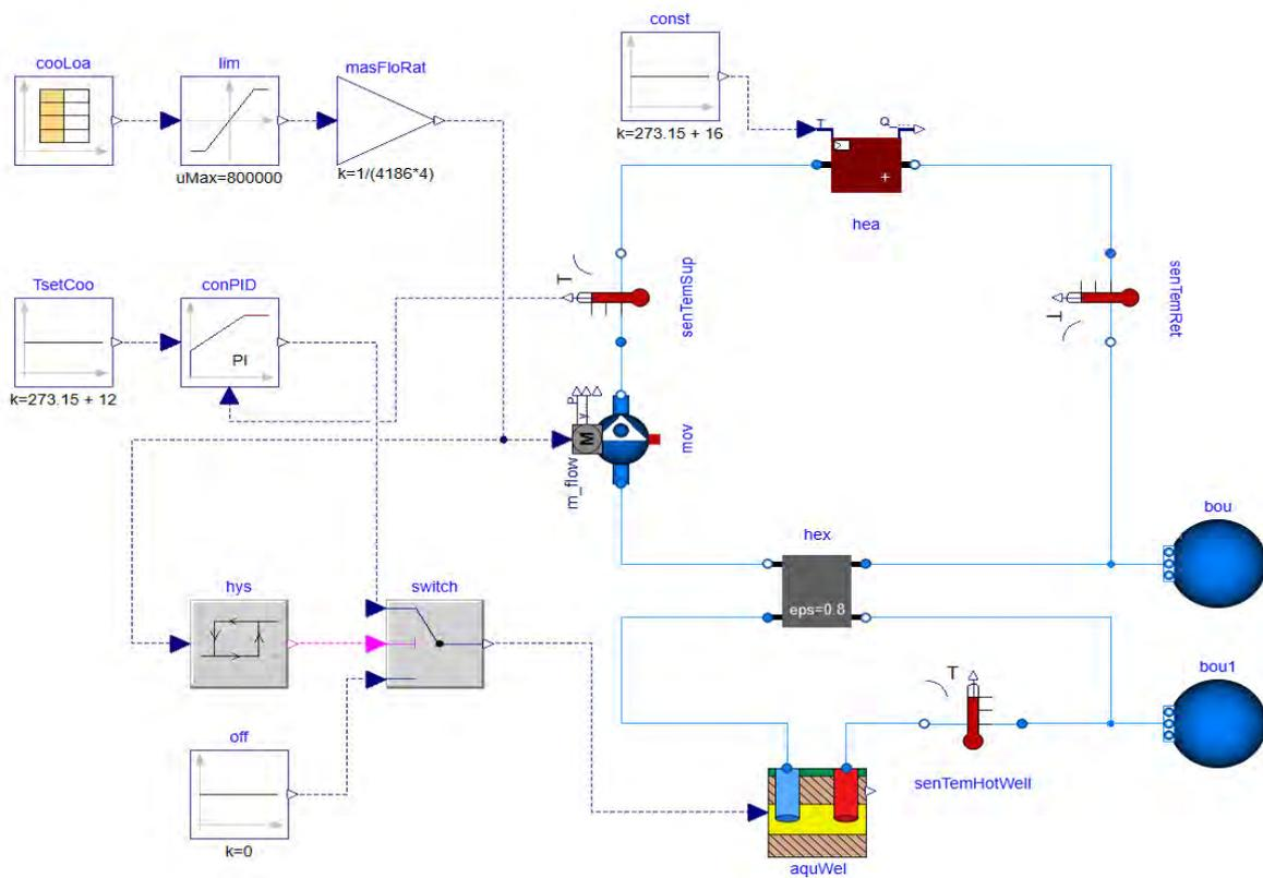
Fig. 2 – Modelica diagram of the ATES system. (The dashed lines represent the control sequence, and the solid lines represent the component connections)
