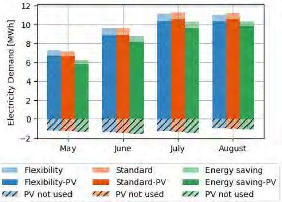
Fig. 5 – Monthly electricity demands of the hotel’s HVAC and DHW systems, with the three-room thermostat strategies. The “-PV” columns represent the net energy demand (considering the PV production instantly used), while the “PV not used” columns represent the energy produced by the PV not instantly used by the system
