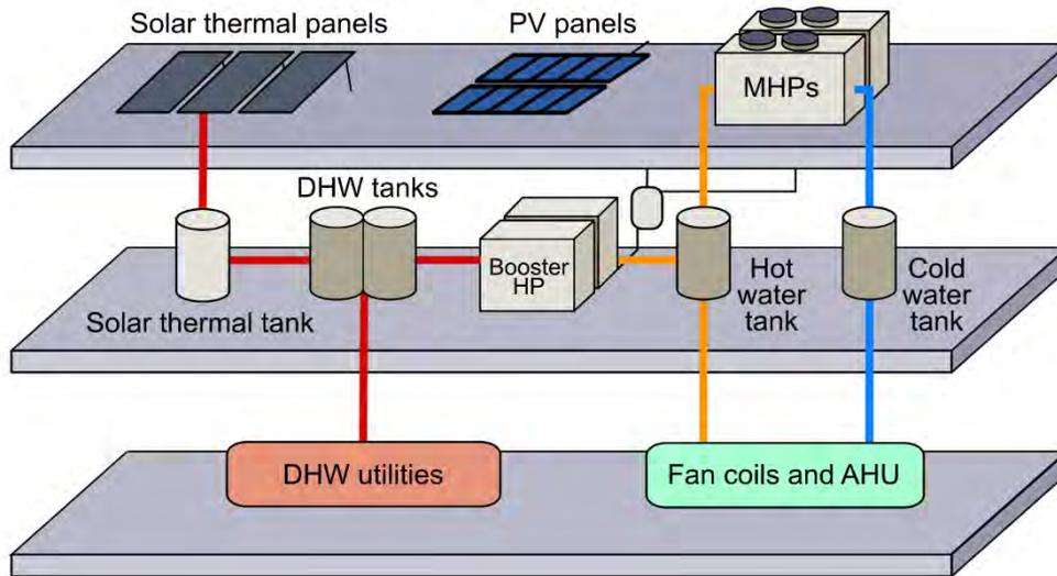
Fig. 2 – HVAC and DHW system scheme
