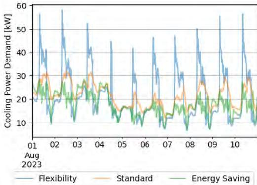
Fig. 3 – Cooling demand calculated with the building simulation with the three studied thermostat strategies (15 minutes timestep). The Flexibility setting allows to reduce the demand in the evenings
