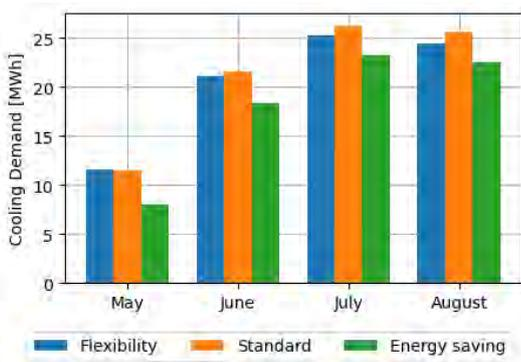
Fig. 4 – Monthly cooling demand calculated with the building simulation with the three studied room thermostat strategies. The “Standard” and “Flexibility” strategies have similar performances
