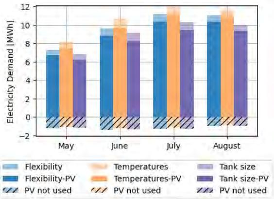
Fig. 6 – Monthly electricity demands of the hotel's HVAC and DHW systems, with the three tank thermostat strategies based on the "Flexibility" cooling demands. The "-PV" columns represent the net energy demand (considering the PV production instantly used), while the "PV not used" columns represent the energy produced by the PV not instantly used by the system
