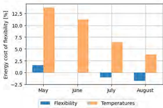
Fig. 7 – Monthly energy cost of flexibility operations of load shifting. The “Temperatures” strategy requires the consumption of more energy during the PV availability to allow the load shifting strategy
