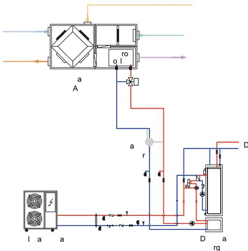
Fig. 2 – Monobloc air source heat pump supplying the domestic AHU and DHW
