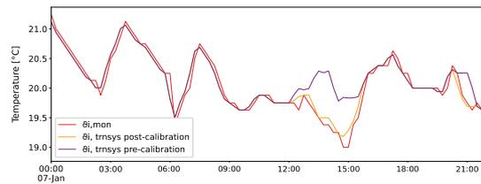
Fig. 4 – Comparison between the set temperature  $\vartheta_{i,mon}$  and the simulated values of the internal temperature pre and post calibration
