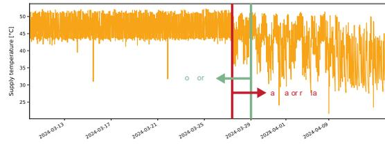
Fig. 6 – Monitored data of the heat pump water supply temperature in the monitored period, before and after the actuator replacement
