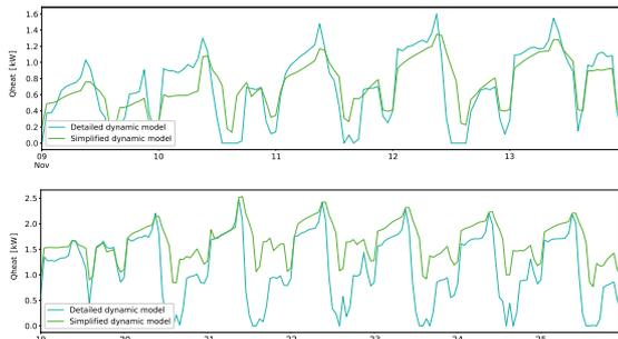
Fig. 8 – Thermal energy demand from simplified dynamic model simulation and from detailed dynamic model simulation on a sample week of November and of January
