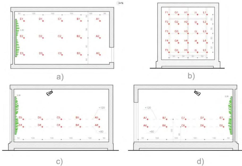
Fig. 2 – Position of the measurements points on horizontal plane (a), ILW surface (b), West side wall (c) and East side wall (d)
