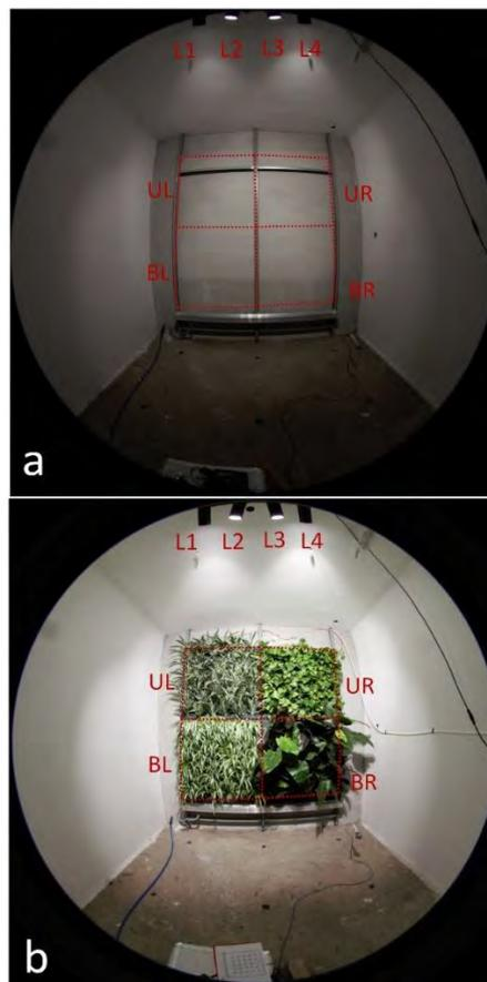
Fig. 1 – View of the ILW within the test cell in  $T_0$  (a) and  $T_1$  (b) through videophotometer
