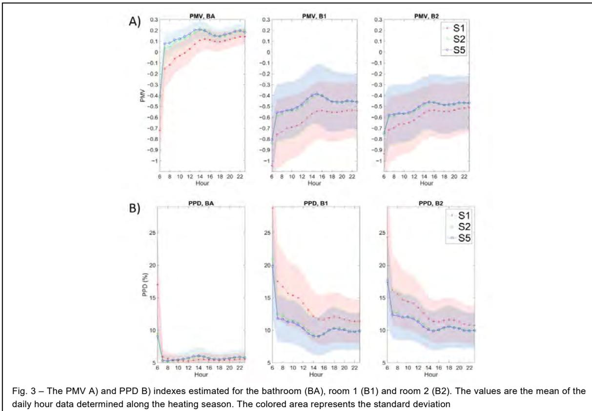
Fig. 3 – The PMV A) and PPD B) indexes estimated for the bathroom (BA), room 1 (B1) and room 2 (B2). The values are the mean of the daily hour data determined along the heating season. The colored area represents the standard deviation
