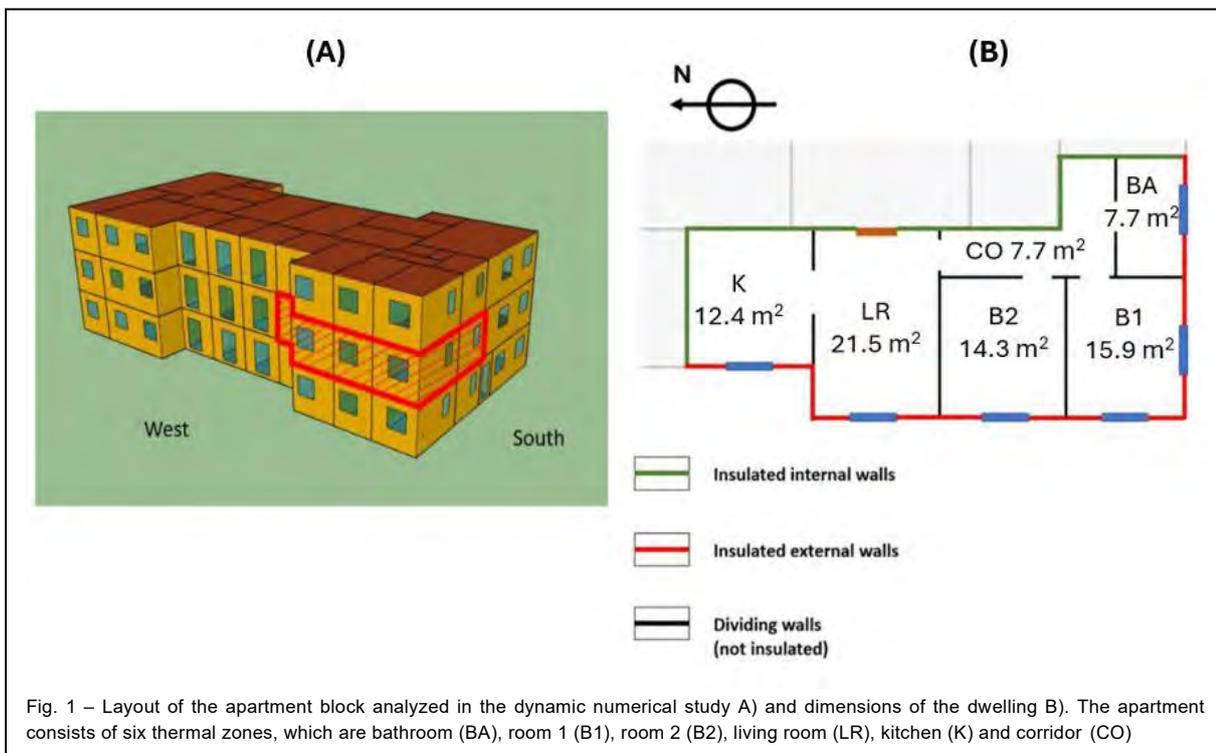
Fig. 1 – Layout of the apartment block analyzed in the dynamic numerical study A) and dimensions of the dwelling B). The apartment consists of six thermal zones, which are bathroom (BA), room 1 (B1), room 2 (B2), living room (LR), kitchen (K) and corridor (CO)
