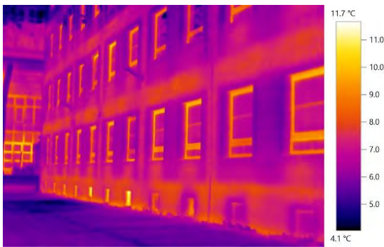
Fig. 3 – Thermal picture of the façade of the ST building
