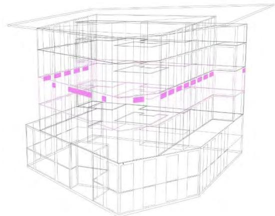
Fig. 10 – Visualization of the optimized louvers integrated into the existing Bullitt Center model in Rhino/Grasshopper, alongside the input data displayed in the Wallacei X Component
