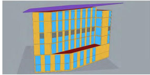
Fig. 4 – View of the existing Bullitt Center modeled in Rhino/Grasshopper with parametric louvers
