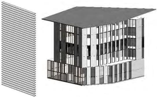
Fig. 3 – View of the existing Bullitt Center modeled in Revit with parametric louvers
