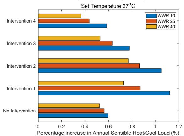
Fig. 14 – Increase in the annual sensible heating/cooling load for set temperature 27 °C
