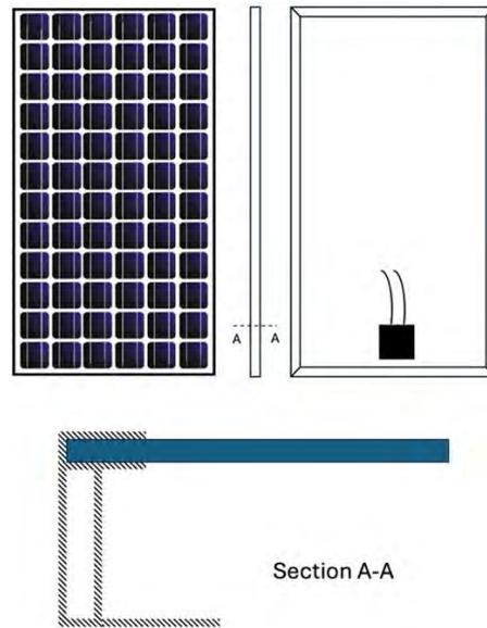
Fig. 3 – A typical commercial c-Si photovoltaic panel construction detail of the edges
