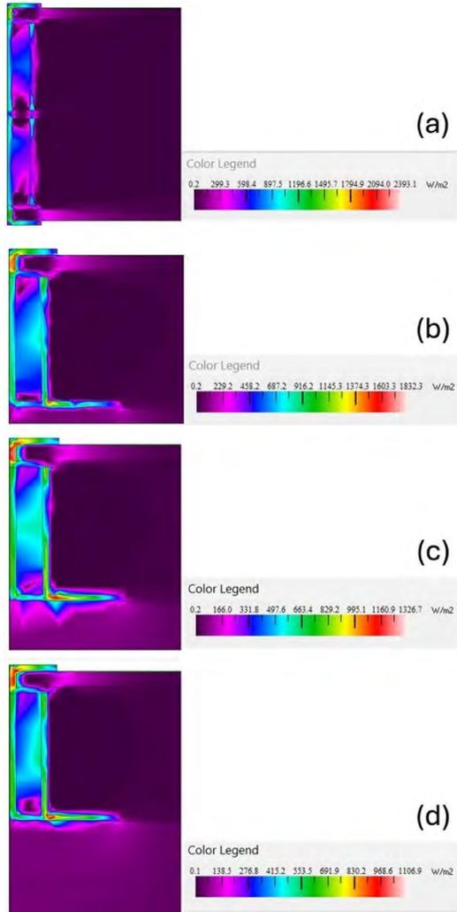
Fig. 9 – Heat flux through PV panel and the frame for the four interventions
