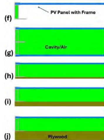
Fig. 6 – Different cases considered for heat transfer analysis with aluminum frame. (f) No intervention, (g) Intervention 1, (h) Intervention 2, (i) Intervention 3, (j) Intervention 4
