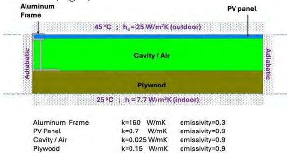
Fig. 4 – Boundary conditions applied to the heat transfer analysis in the THERM tool
