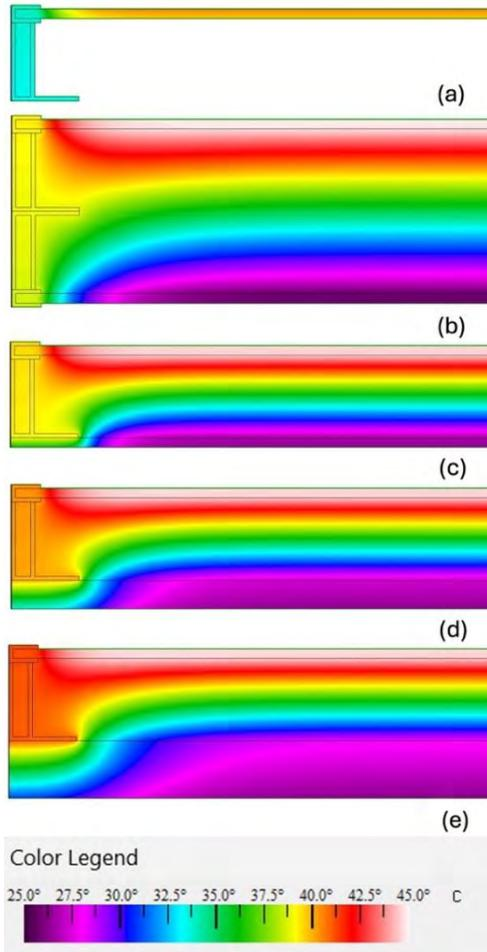
Fig. 7 – Temperature profile of the PV cross-section for different cases
