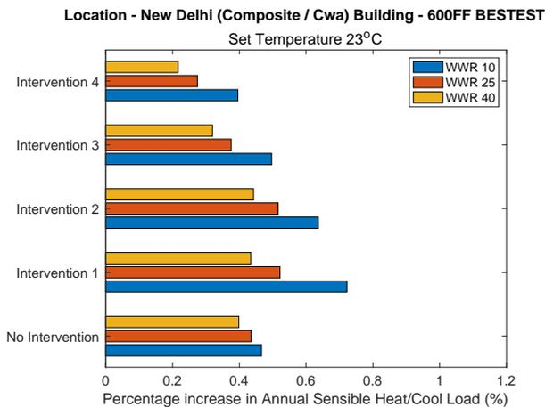
Fig. 12 – Increase in the annual sensible heating/cooling load for set temperature 23 °C
