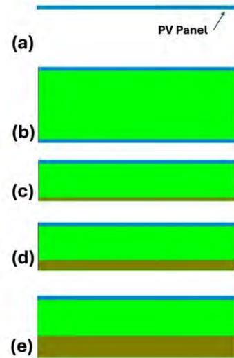
Fig. 5 – Different cases considered for heat transfer analysis without aluminum frame. (a) No intervention, (b) Intervention 1, (c) Intervention 2, (d) Intervention 3, (e) Intervention 4
