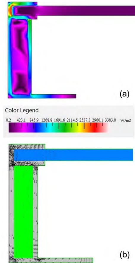
Fig. 8 – Heat flux through PV panel and the frame
