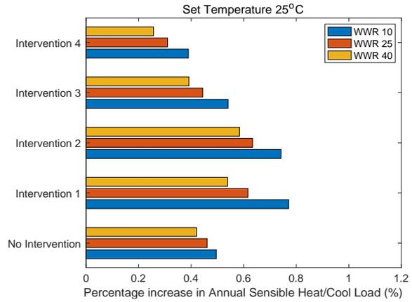
Fig. 13 – Increase in the annual sensible heating/cooling load for set temperature 25 °C
