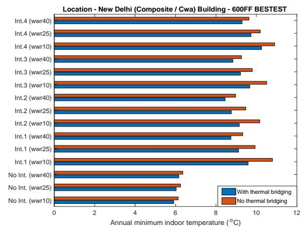
Fig. 10 – Annual minimum indoor air temperature with and without thermal bridging effects
