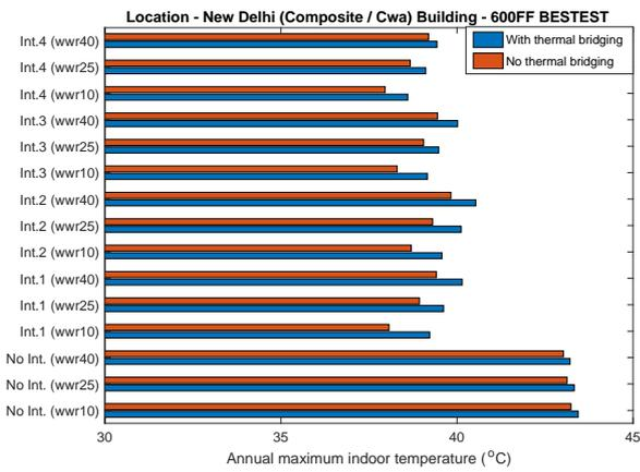
Fig. 11 – Annual maximum indoor air temperature with and without thermal bridging effects
