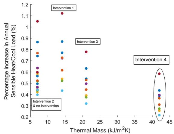
Fig. 15 – Desirable intervention considering thermal mass and thermal bridging effects
